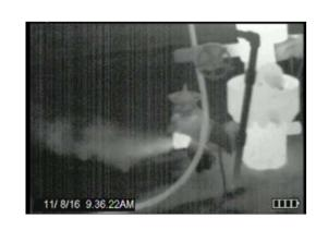
Leak from a wellhead
