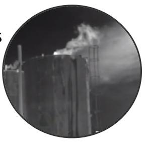
Methane from a storage tank « seen » with an infrared camera
